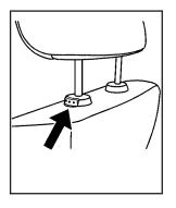
Pull the restraint up to raise it. To lower the head restraint, press the button, located on the top of the seatback, and push the restraint down.
